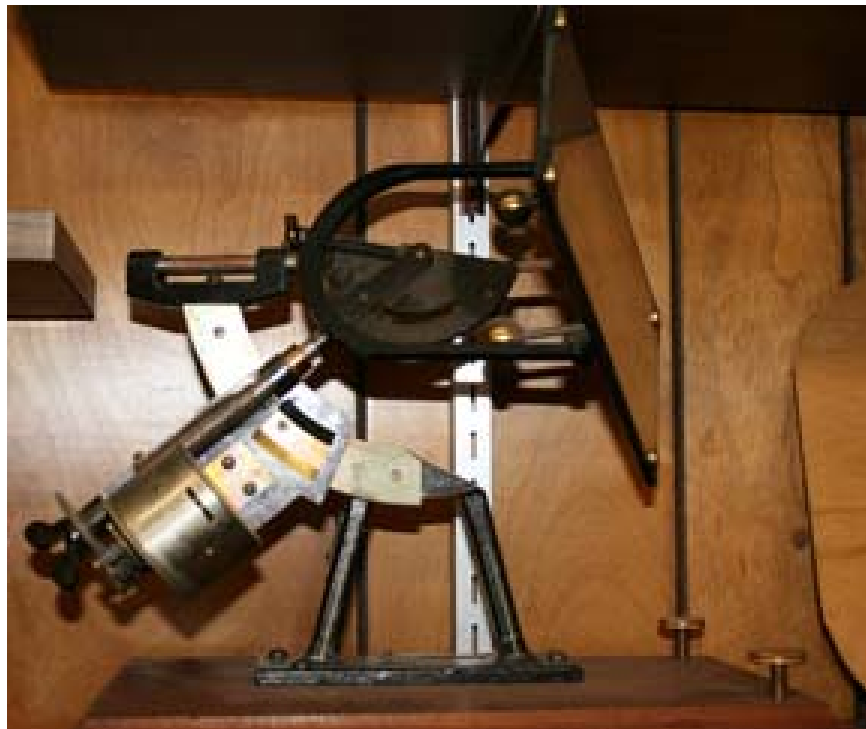
Sunlight microscope illuminator, invented by AE Douglass (ca. 12 inches tall).
