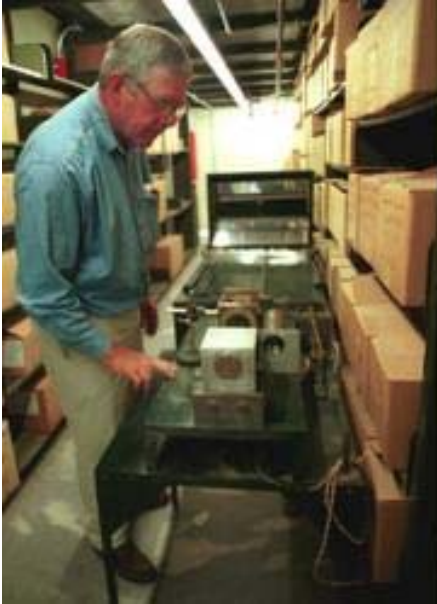
AE Douglass' cycloscope - a tool invented and used by him in a long but ultimately unsuccessful quest to discover cycles of solar activity in tree rings. (curated by ASM; see http://uanews.org/node/8105 )
