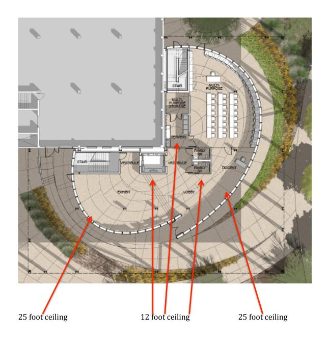
Note: for scale, the black vertical "I-beams" shown in the exhibit floor are spaced at 12 feet apart.
