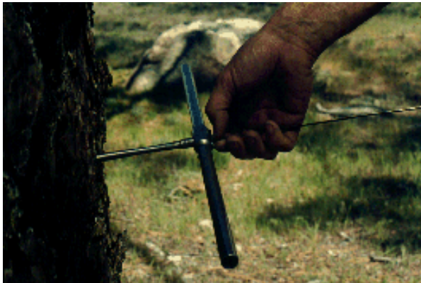
Figure 18. A researcher is coring a tree using increment borer.
