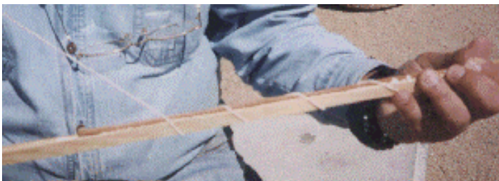
Figure 23. Wrapping the core with a string to hold the core in place until the glue is dry.
