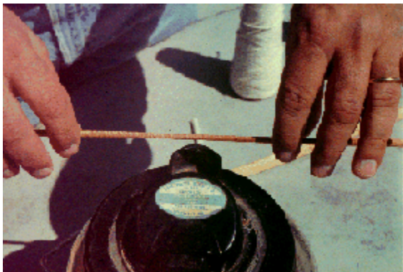
Figure 20. Straightening a twisted core over a jet of steam.
