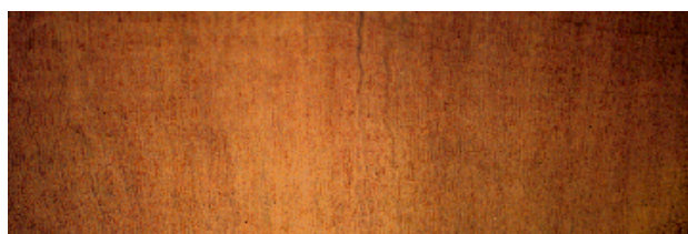
Figure 27. Before sanding the sample. Notice that the ring boundaries are not distinct.
