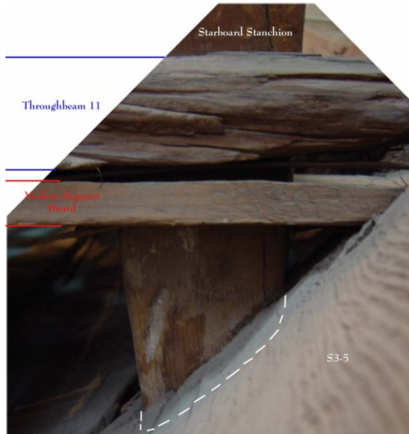
Figure 52. Starboard quarter rudder stanchion socket, GC 4926 (P. Creasman).
