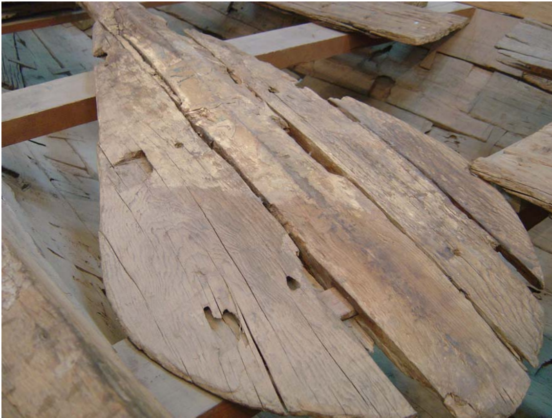
Figure 29. Blade of a quarter rudder (J. Levin).
