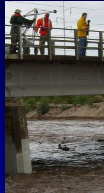
Taking a discharge measurement during a flood
