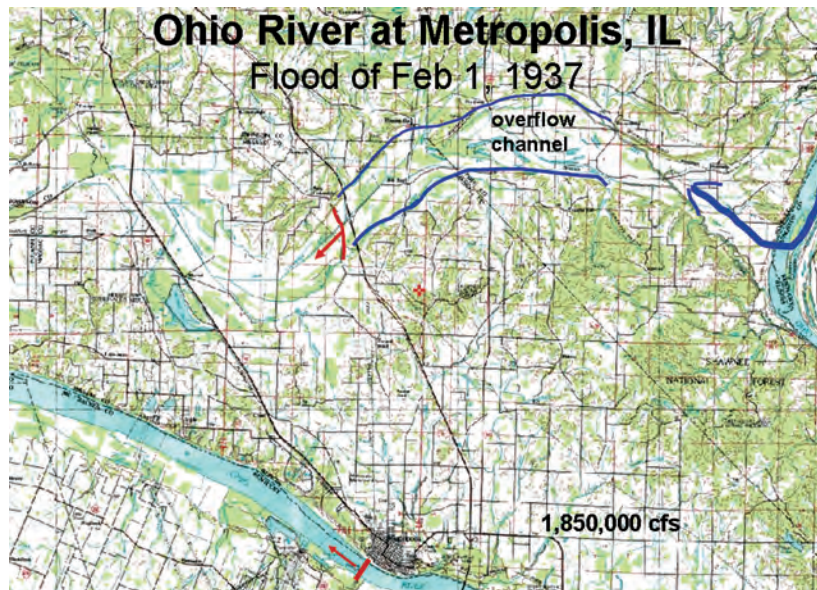
Figure 34. Location of overflow channel for 1937 flood on the Ohio River at Metropolis, Illinois. Arrows mark place when the floodwater left the main channel, and the path of the overflow.
