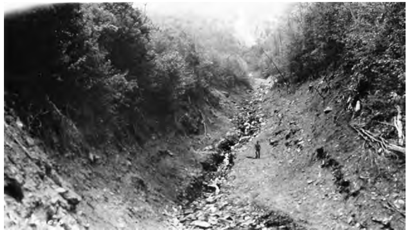
Figure 5. View looking upstream of slope-area measurement site after storm of August 1940, Big Creek, North Carolina. Note person in right-center of photograph for scale and the U-shaped channel cross-section characteristic of some debris-flow channels.
