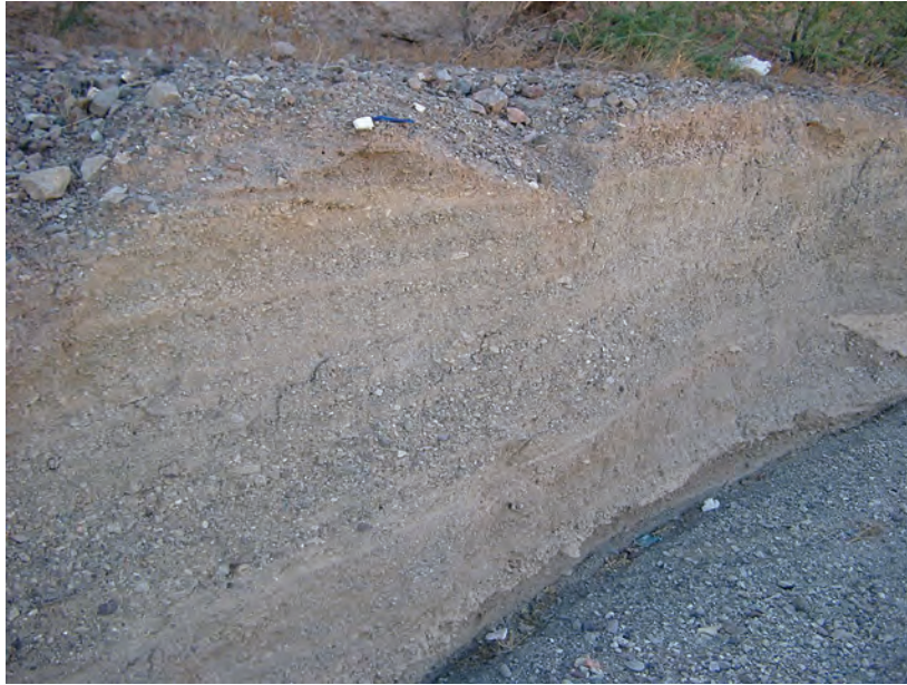
Figure 25. Stratigraphy of terrace in slope-area reach of Eldorado Canyon at Nelson Landing, Nevada, showing clear stratification associated with fluvial depositional processes and not originating from debris flows, August 2003.
