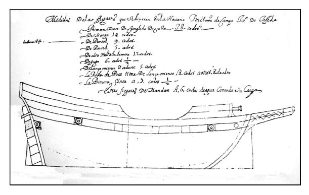
Figure 4. Depiction and principle dimensions of a *fragata* built under the direction of Juan de Tejada in Havana, ca. 1600. *Archivo General Simancas; Mapas, Planos y Dibujos* 42, 70; published in Otero Lana 1991: 90
