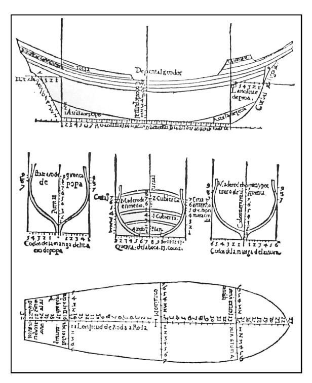
Figure 3. García de Palacio's *galeoncete*-like ship (*nao*) of 150 *toneladas*, from the *Instrucción náutica* published in Mexico City, 1587. Top: Longitudinal or sheer profile (compare with the *fragata* in Figure 4). Middle: Hull sections at the stern, midships or master frame, and bow. Bottom: Plan view of lower deck (note some of its labels are printed backwards). From García 1944 [1587]: 96-97.
