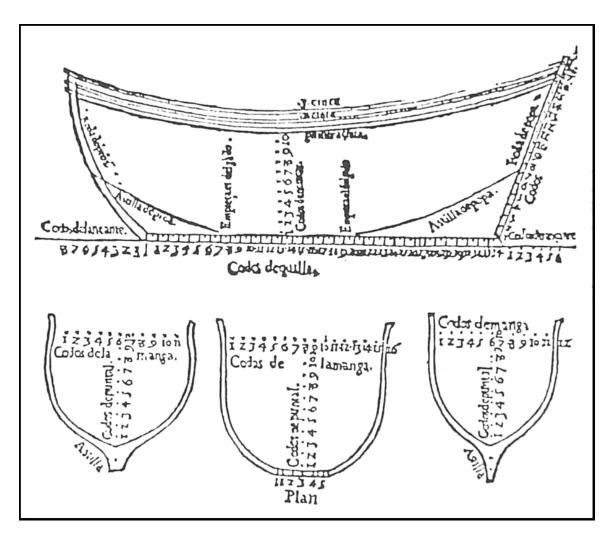
Figure 2. García de Palacio's *nao* of 400 *toneladas*, from the *Instrucción náutica* published in Mexico City, 1587. Longitudinal or sheer profile is above (note the flush profile or lack of raised superstructure); below are hull sections at the bow, midships or master frame, and stern. The dimensions of this ship are listed in Table 1. From García 1944 [1587]: 93-94.
