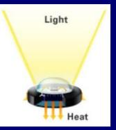
LED bulbs use light emitting diodes to produce light. The movement of electrons through a semiconductor material illuminates the tiny LED light sources. A small amount of heat is released backwards, into a heat sink.
