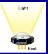
LED bulbs use light emitting diodes to produce light. The movement of electrons through a semiconductor material illuminates the tiny LED light sources. A small amount of heat is released backwards, into a heat sink.
