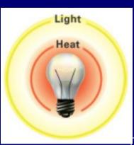
**Incandescent bulbs** create light by passing electricity through a metal filament until it becomes so hot that it glows.
