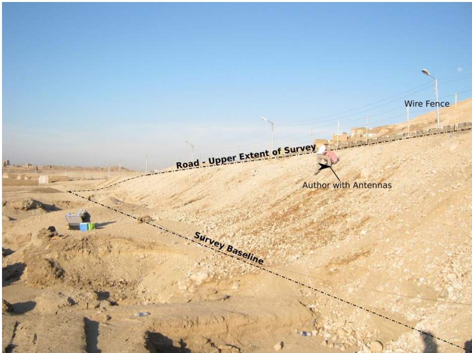
Figure 10-2: A view of the road embankment looking south. The author is holding the radar antennas in place during data acquisition on the slope. The steel fence and buried utilities are potential sources of interference.
