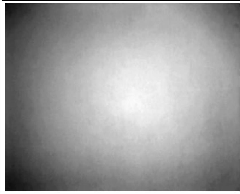
FIGURE 3.5. Example of illumination nonuniformity. The center-to-corner difference in graylevel is about 25%.
