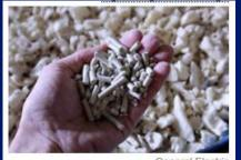
The refrigerator's foam insulation is turned into pellets that can be used as fuel.
